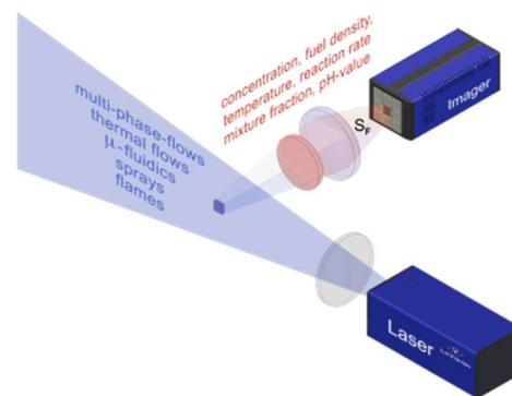
Figure 2: Laser induced fluorescence (LIF); Source: LaVision
