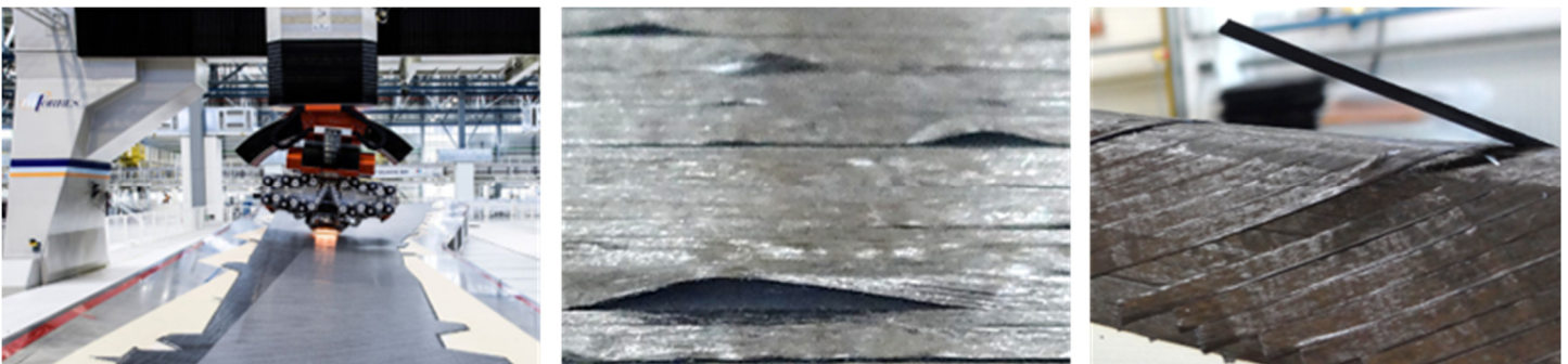
Figure: Automated Fiber Placement [Airbus] (left), lay-up defect out-of-plane buckling (middle), lay-up defect tape peel-off (right)
