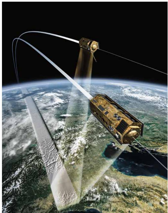
**The twin satellites TerraSAR-X and TanDEM-X** orbiting Earth at an altitude of around 500 kilometers. The TanDEM-X mission will survey all 150 million square kilometres of Earth's land surface several times over during its three-year mission, delivering a global elevation model that is homogeneous in quality and unprecedented in accuracy. It produces 3 petabytes of data and one trillion data points, each representing an area of 12 m<sup>2</sup> at a height accuracy of 2 meters.
