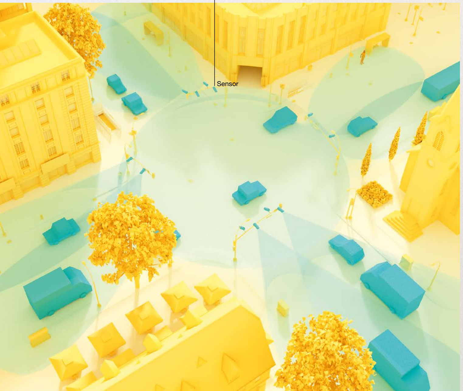
Camera image superimposed with lidar data (coloured point cloud)
