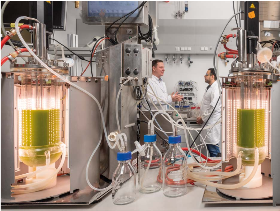
Laboratory scaling of algae cultivation in closed photobioreactors. The technical data generated here are the basis for the next process scale-up steps at the TUM AlgaeTech Center in Ottobrunn.
