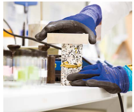
After joining of the granite test specimens, they are loaded with 2 kg of weight until the hot-melt adhesive has cooled down.
