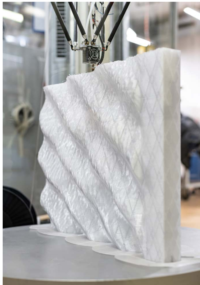
3D printing of a facade element (ca. 80x90 cm) at the technical center of the TUM Department of Architecture. The printer is a large area delta printer.
