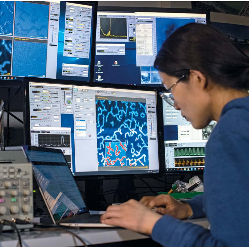
△ PhD candidate Nan Cao works at the scanning tunneling microscope. The screens show STM images featuring chain-like covalently bonded molecular structures (white/light blue) grown on a gold surface (dark blue). Selected molecular chains are highlighted in red.
