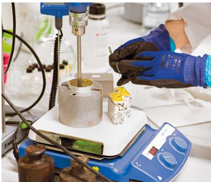
After applying hot-melt adhesive to the heated granite test specimens, glass beads of 400 µm in size are scattered on the bonding surface to achieve a constant reproducible joint thickness.
