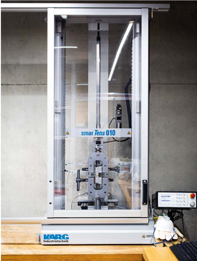
Universal testing machine for the determination of tensile lap-shear strength of bonded assemblies.
