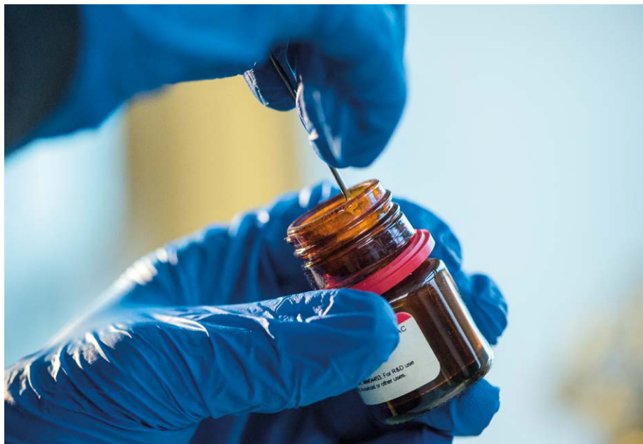
Preparatory steps to evaporate molecules onto the surface: Cobalt-phthalocyanine molecules are transferred from the container into a quartz crucible.
