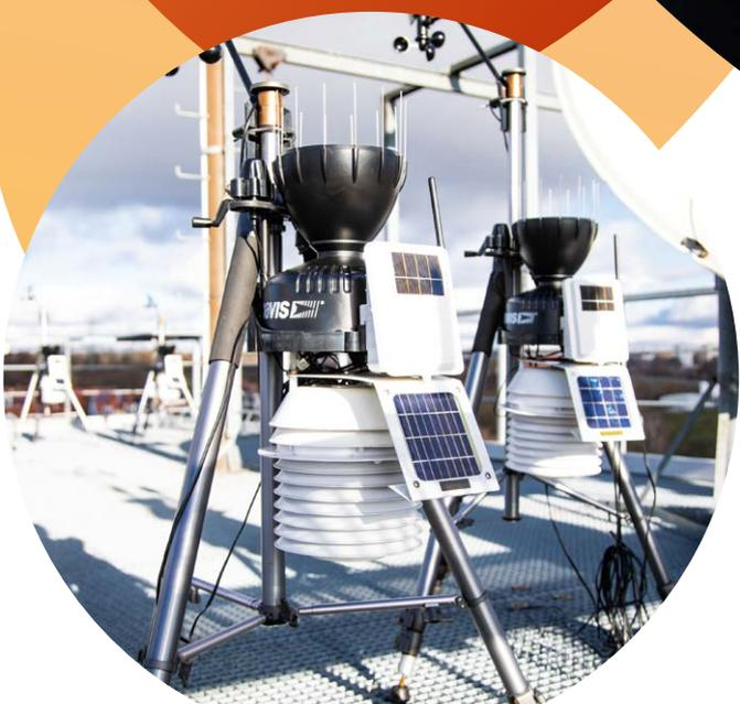
**A rooftop meteorological station**, high above the TUM School of Life Sciences Campus, is used for measurements and for testing measurement equipment before field use.
