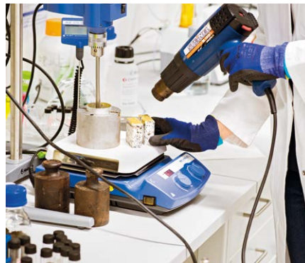
The adhesive-coated bonding surfaces are heated using a heat gun before joining.
