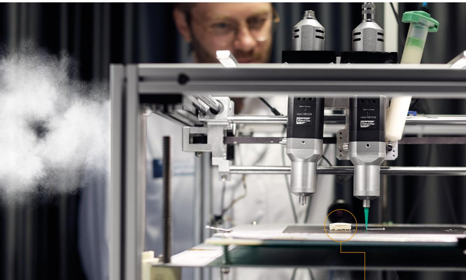
The researchers have been working to investigate the printability of dough and optimize the process for three years. “Applying the dough evenly represented a major challenge: The tough, elastic mass of flour and water needs to be squeezed through a funnel, the deposition, without the narrow opening of barely a millimeter wide becoming blocked,” explains Jekle, the Head of the Chair’s Cereal Technology and Process Engineering research group.
