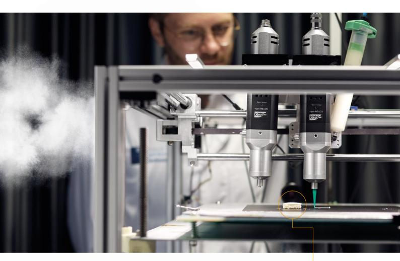
The researchers have been working to investigate the printability of dough and optimize the process for three years. "Applying the dough evenly represented a major challenge: The tough, elastic mass of flour and water needs to be squeezed through a funnel, the deposition, without the narrow opening of barely a millimeter wide becoming blocked," explains Jekle, the Head of the Chair's Cereal Technology and Process Engineering research group.
