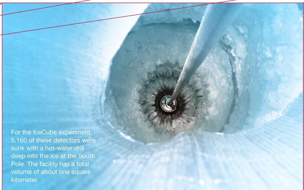
For the IceCube experiment, 5,160 of these detectors were sunk with a hot-water drill deep into the ice at the South Pole. The facility has a total volume of about one square kilometer.
