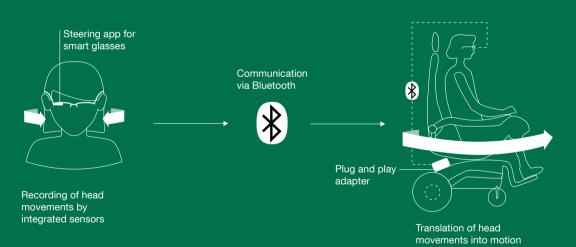
Munveo's control solution can be easily adapted to electric wheelchairs. It uses smart glasses to detect the wearer's head movements. The data is sent via Bluetooth to a special adapter, which then translates this information into motion commands.
