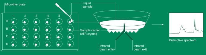
The core component of the ATR (attenuated total reflectance) infrared sprectroscopy technique is the crystal, which is used as a sample carrier and reflects the infrared light. The IRUBIS team has developed a low-cost silicon crystal with high sensitivity. Integrating many crystals into a well plate can make it possible to investigate up to 96 measurements simultaneously.
