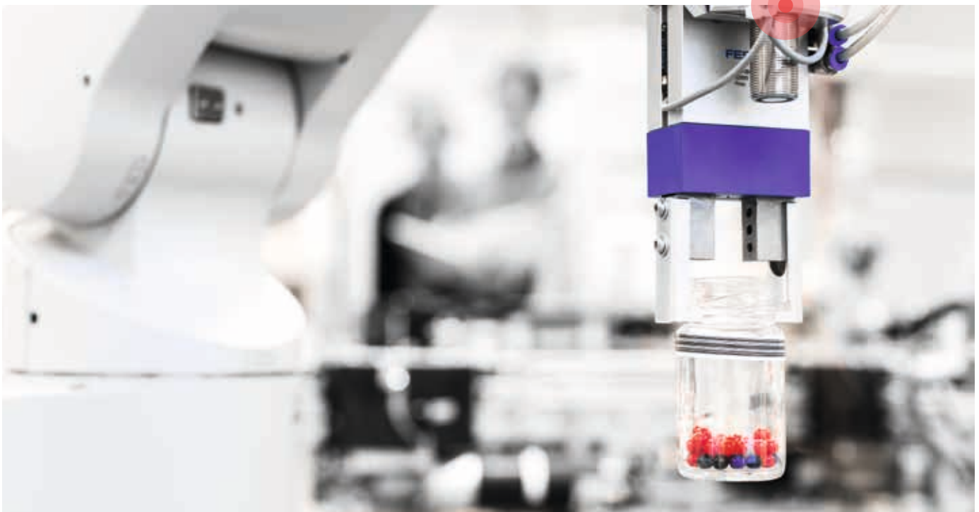
Robotic arm picks up containers and places them onto belt
