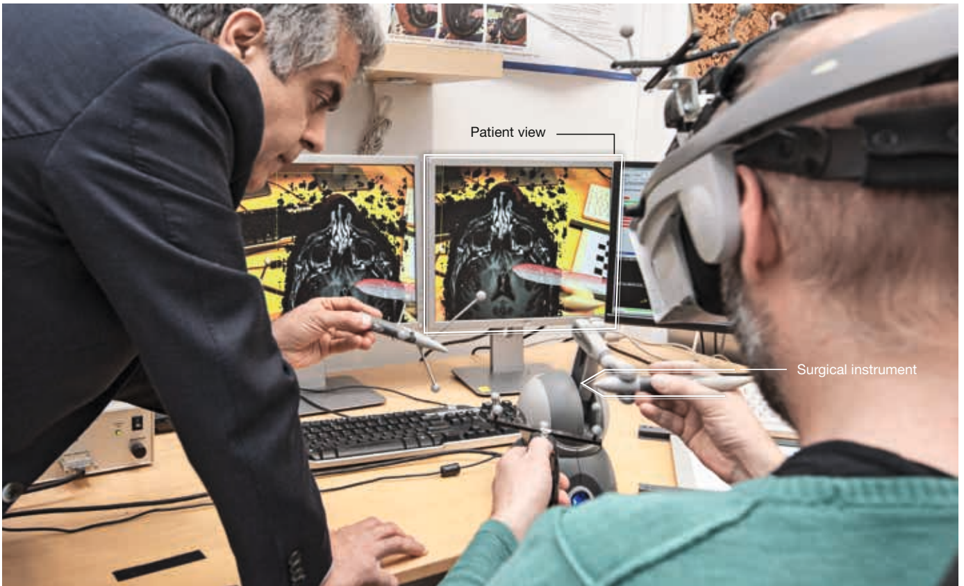
Tests with a see-through augmented reality HMD: While cameras on the HMD allow for the augmentation of the patient view, infrared markers allow the HMD to be localized and co-registered with surgical instruments. Co-registration means that position and orientation of real and virtual objects match.
