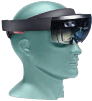
Augmented reality optical see-through headsets have a transparent display and overlay the reality that the user views through the glasses with additional information.
