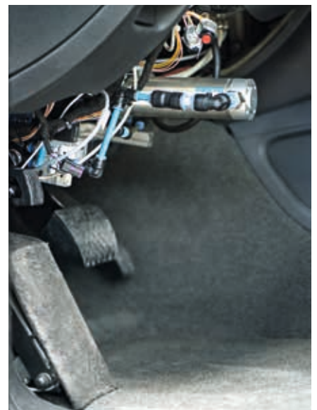
Camera systems record the front and side view from the cockpit. All images are transmitted via mobile communication to the operator, who controls the steering wheel and pedals.
