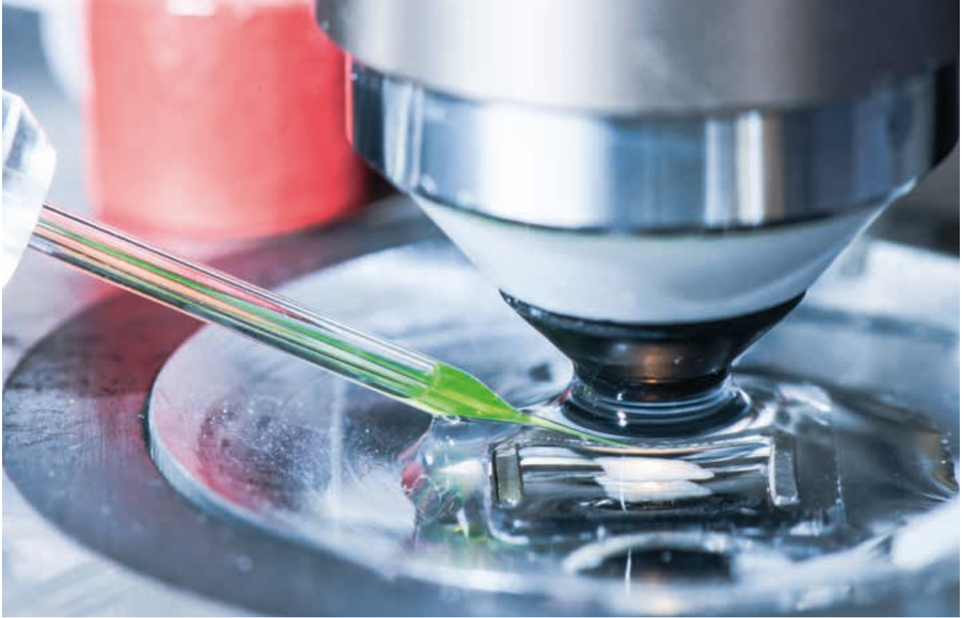
Konnerth's working group combines patch clamp measurements , which involve attaching a pipette onto the nerve cell by suction, with two-photon microscopy. The micropipettes are fabricated internally by the group.
