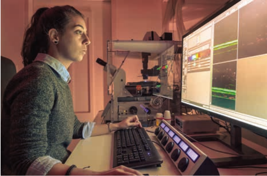
Maria Cunha, a Ph.D. student in Simons' laboratory, uses a confocal microscope to observe myelination in a living but sedated zebrafish (inside the petri dish in the lower image).
