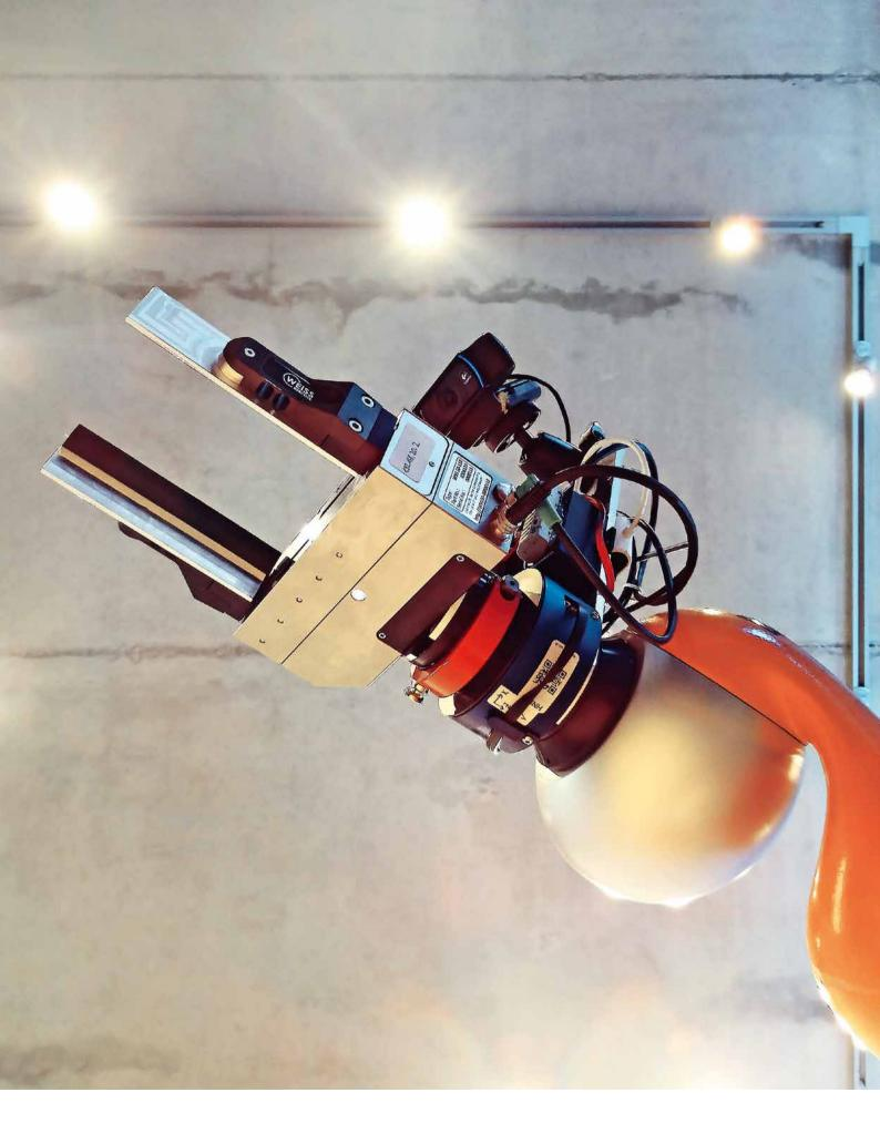
A low cost robot gripper with precision: The ROVI system employs gripper jaws made of rubber. When it grips an object, the rubber is compressed and a camera registers this deformation.
