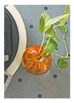
When the robot encounters an object, the ROVI system detemines whether measured force can be applied to move the item out of the way or whether the robot needs to navigate its way around it.
