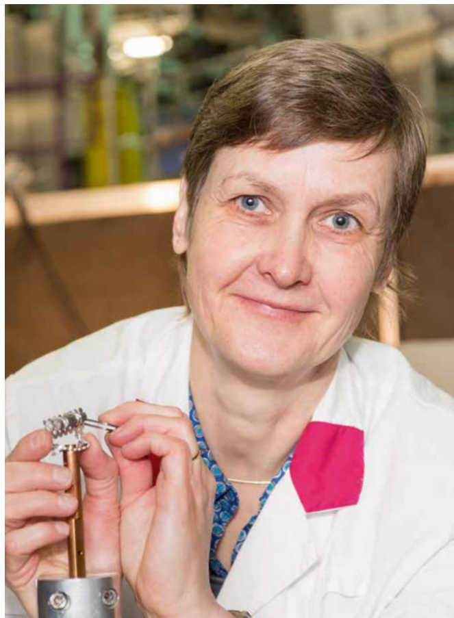
Astrid Schneidewind mounts a high temperature superconductor sample for the neutron scattering experiment. During the measurement itself, the sample is positioned in a cryostat and people are not allowed near the experiment.
