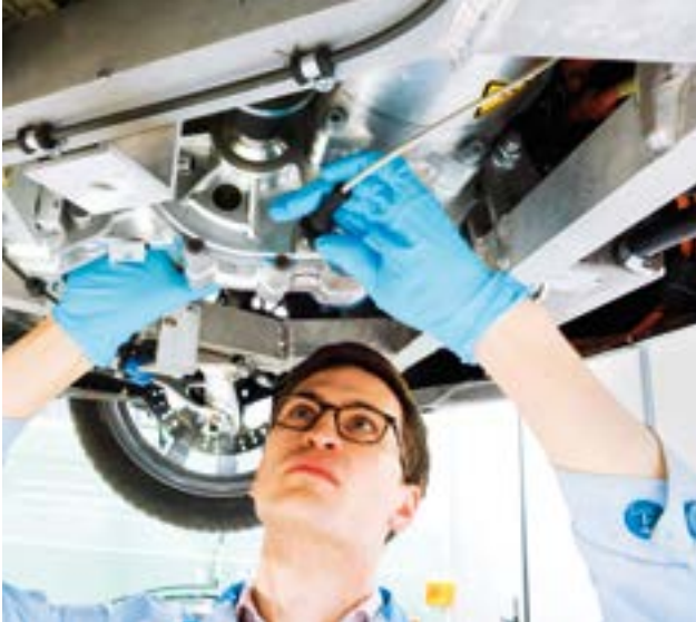
In the workshop of TUM's Institute of Automotive Technology: The torque vectoring drive installed in the Visio.M electric vehicle (left page). Philipp Gwinner connects one of the sensors (top) to the drive.
