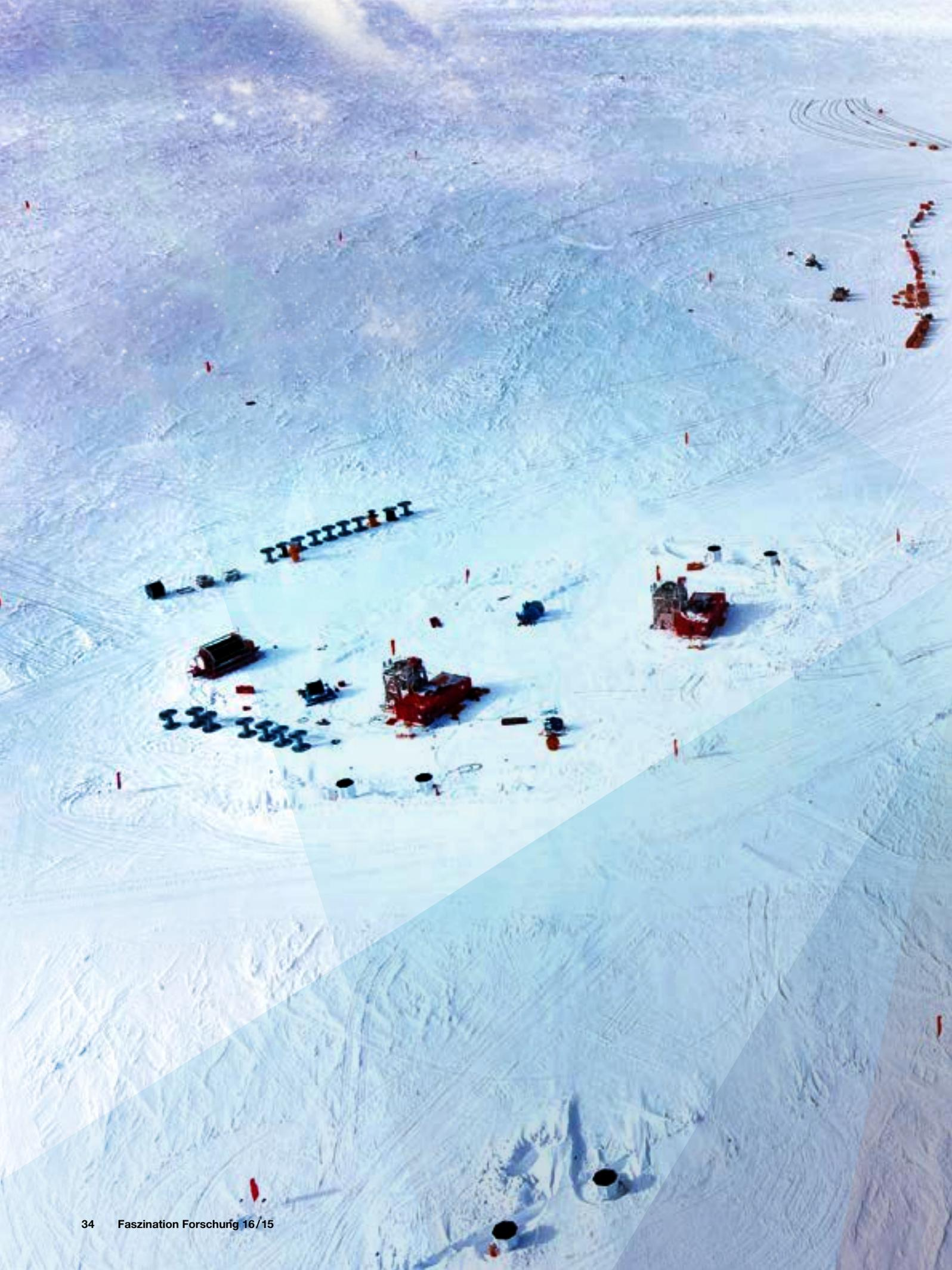
**An aerial view** of the IceCube Lab. To the left of the lab are drilling hoses, towers and equipment, to the back right is the seasonal equipment site. The lab covers a surface of 1 square kilometer.
