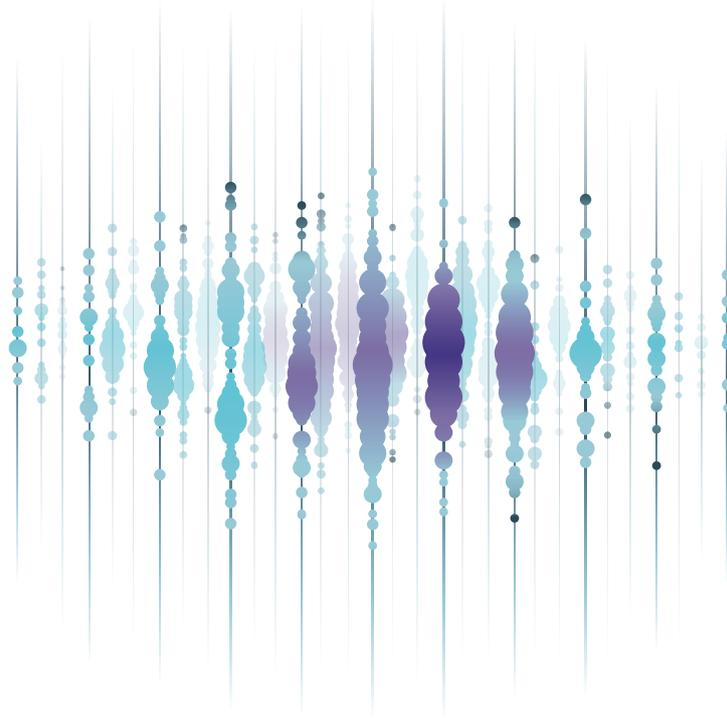
**A neutrino observed in IceCube:** The colored spheres indicate optical sensors that detected light. The color corresponds to the arrival time of the light signal. Red marks the beginning, light blue the end of the event, which typically lasts a few microseconds. The size of the colored spheres corresponds to the amount of detected light.
