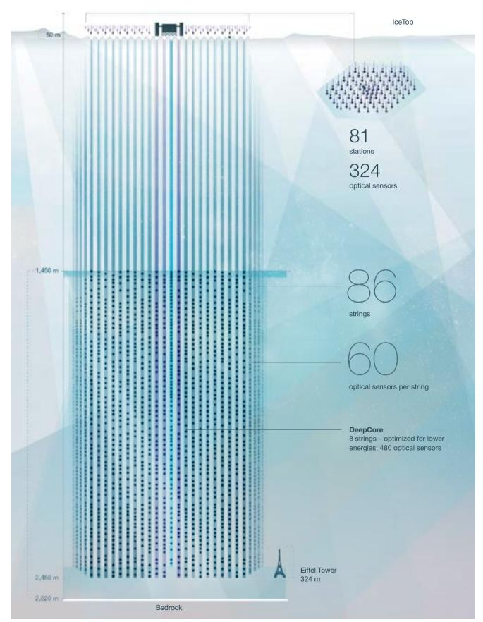
**The IceCube Neutrino Observatory** is the world's largest neutrino detector. Located at the South Pole, IceCube is buried inside the ice masses of Antarctica, reaching a depth of about 2,500 meters. In total, it encompasses a cubic kilometer of ice. IceCube is made up of 5,160 light sensors attached to 86 vertical strings spaced at intervals of 125 meters. The sensors collect light emitted by particles that are produced during interactions between neutrinos and ice molecules.
