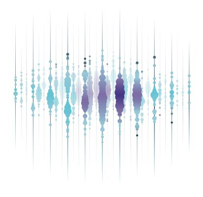
A neutrino observed in IceCube: The colored spheres indicate optical sensors that detected light. The color corresponds to the arrival time of the light signal. Red marks the beginning, light blue the end of the event, which typically lasts a few microseconds. The size of the colored spheres corresponds to the amount of detected light.
