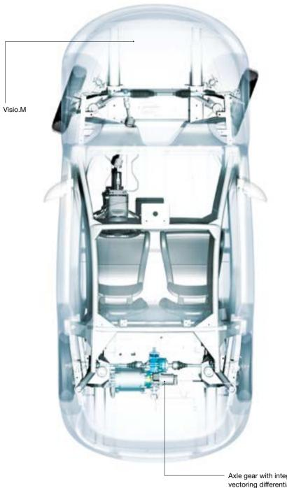
Axle gear with integrated torque vectoring differential
