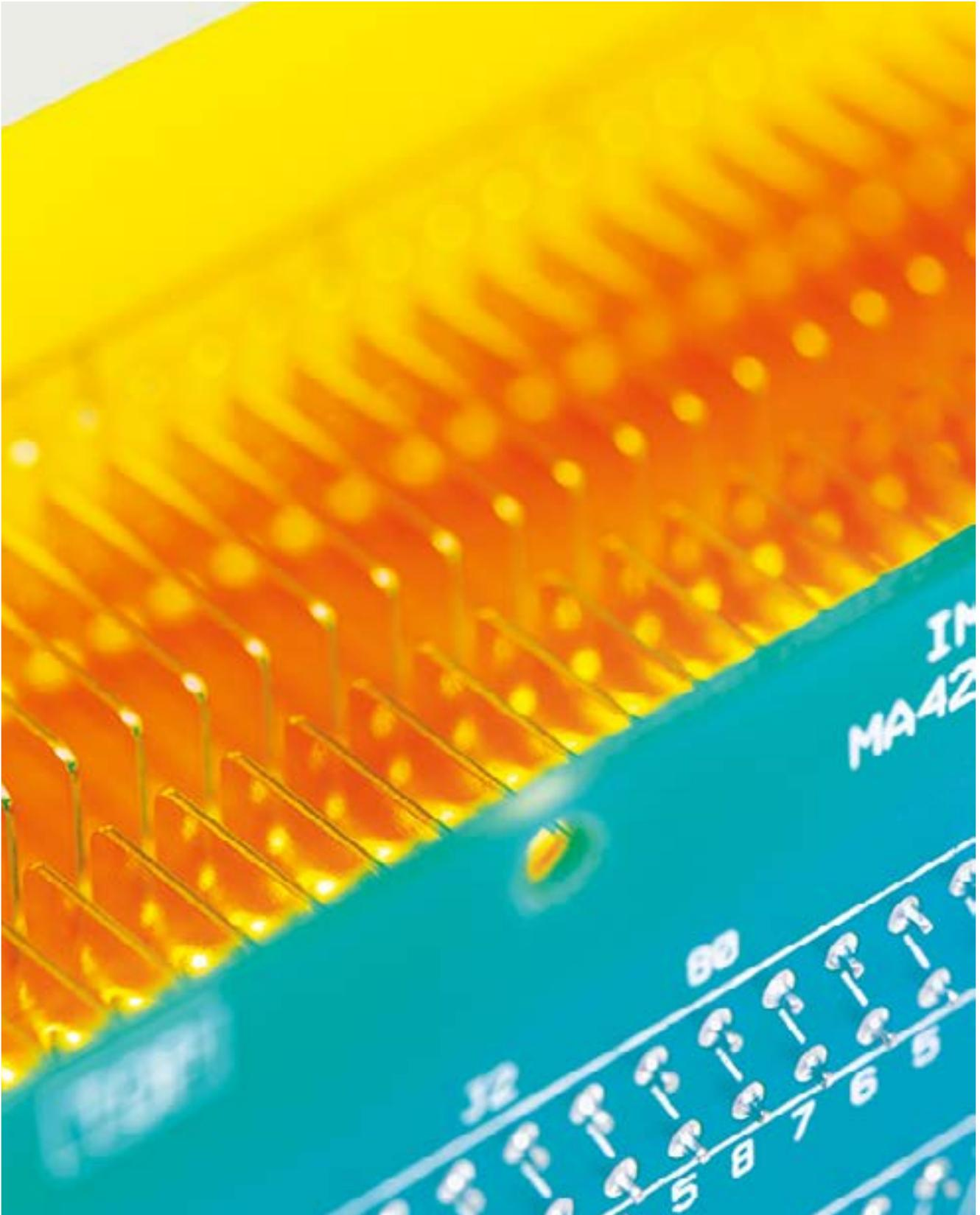
**Inside the mass spectrometer**, the ions are accelerated. The resulting ion beam enters a magnetic field, which deflects the individual ions according to their mass and charge. The above image shows a so-called stacked electrode, which is part of the optics that focus the ion beam.
