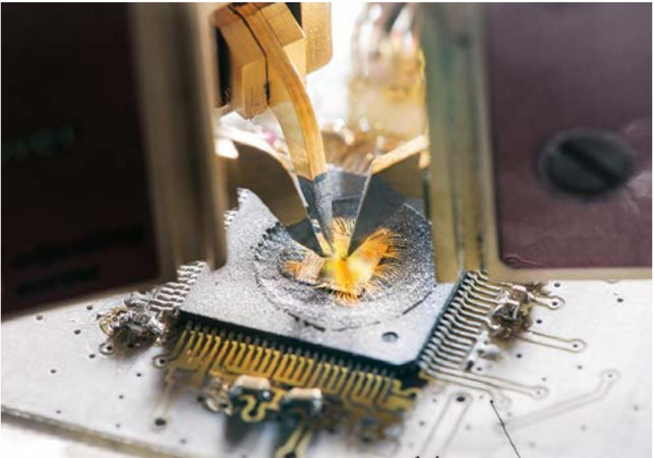
**Chips under attack in Georg Sigl's laboratory:** Measuring electromagnetic radiation to prepare for side channel attacks (top left); fault injection with power glitches in order to perform fault attacks (top center); firing laser beams at an open processor chip while it carries out calculations. The laser causes calculation failures, which can be used to extract secret information (top right). Side channel attack by means of three highly sensitive measuring probes (bottom).
