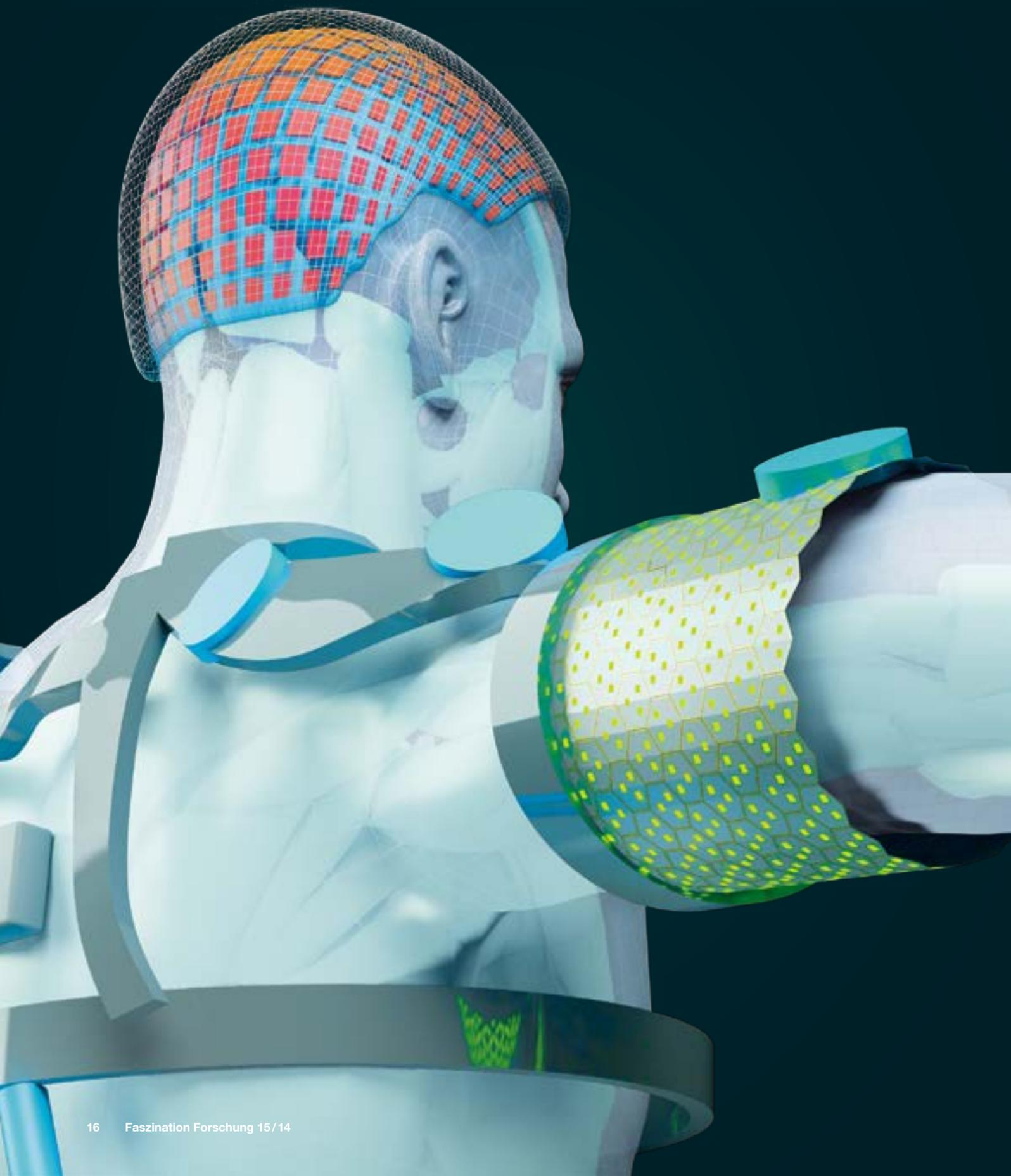
**The Walk Again Project** aims to overcome paralysis with the help of a phenomenal amount of smart technology. It utilizes an exoskeleton controlled by the thought of a paralyzed person. An electrode cap detects the brain signals, and a computer integrated into the suit converts these into commands for movement.
