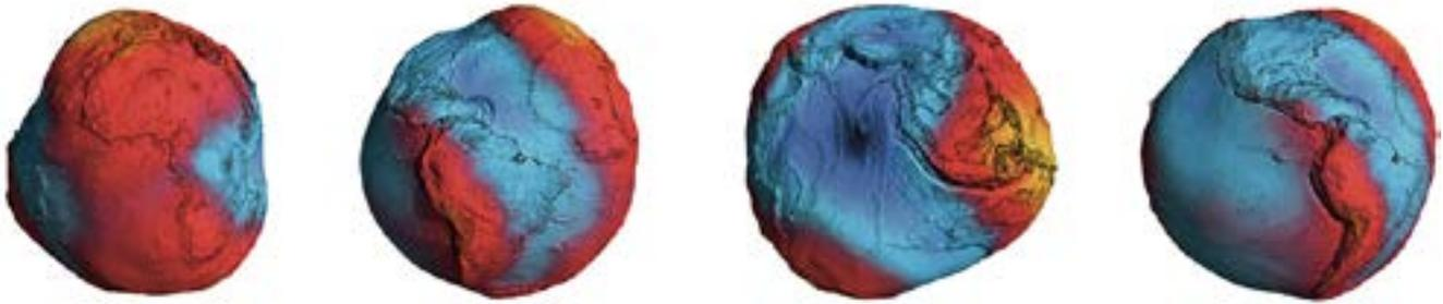
**Earth in the “light” of gravity:** These four views show the height of the geoid — which corresponds to the mean ocean surface at rest — above or below a reference model for Earth’s shape that is based not on gravity, but on the planet’s rotation. Deviations above (red) or below (blue) the reference surface are caused by mass anomalies in Earth’s mantle.
