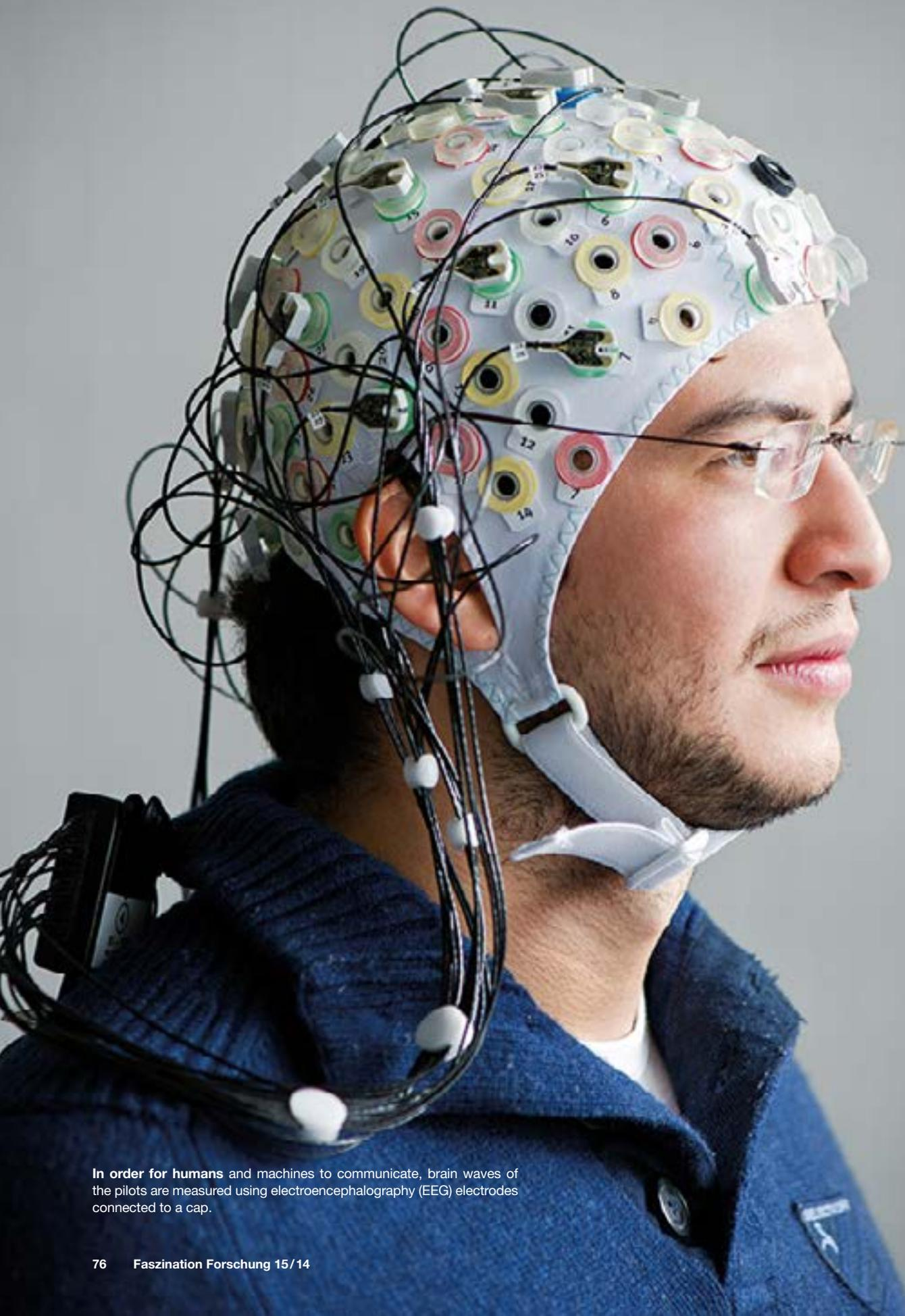
In order for humans and machines to communicate, brain waves of the pilots are measured using electroencephalography (EEG) electrodes connected to a cap.
