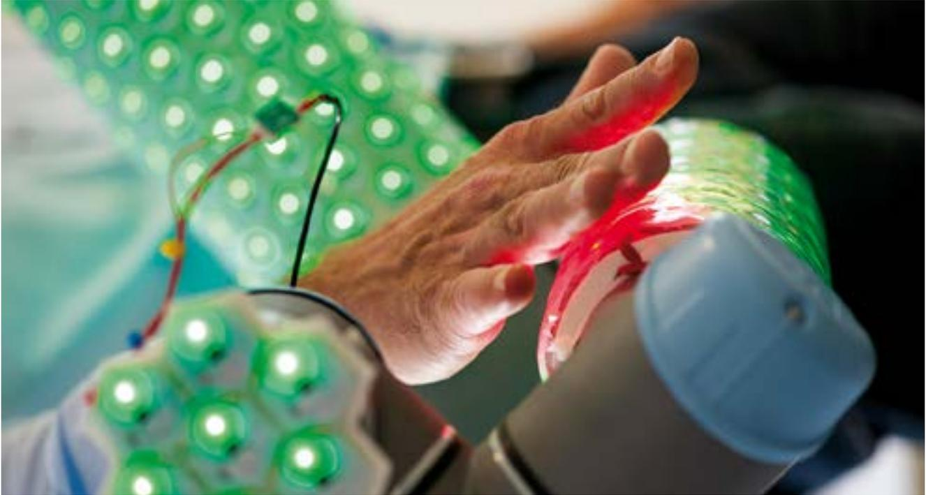
**Touching the artificial skin of a robot part.** The multimodal-cellular skin is named CelluARSkin. It consists of several hexagonally shaped unit cells, each featuring multiple sensor modalities. The artificial skin makes it possible to enrich robot interactions through a multimodal sense of touch.
