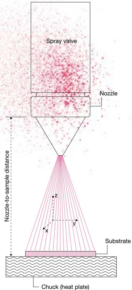
**The basic principle of the high-tech spray nozzle** is not unlike conventional air brushing. But here, everything must be perfect to ensure that extremely thin layers can be applied evenly. The Munich-based researchers have become adept at producing homogeneous inks from the exotic substances, adhering them to the substrate and achieving a perfectly even spray film.
