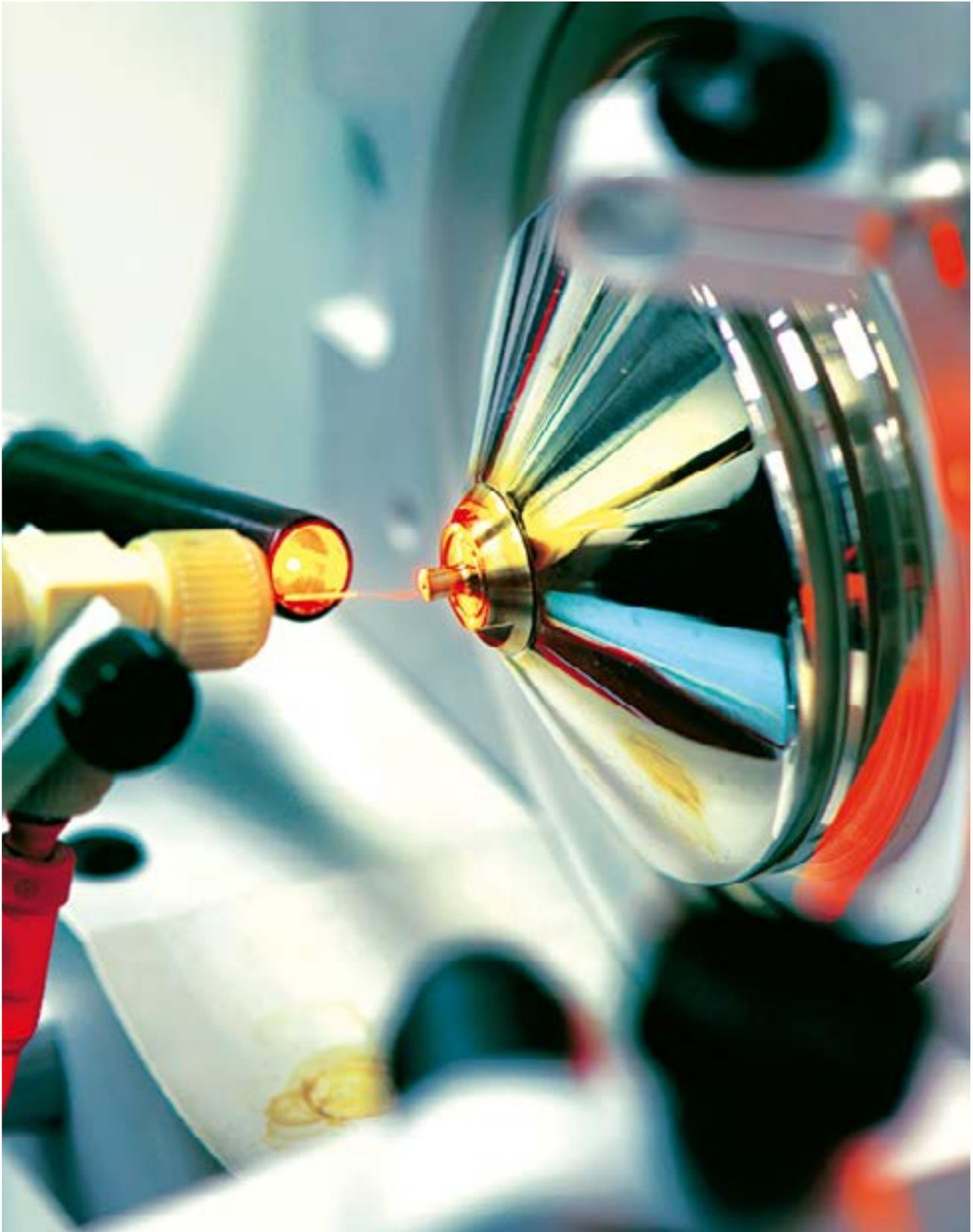
**Ionizing peptide samples for mass spectrometry.** Guided via a thin glass capillary (left), the samples encounter high electric voltage and are transferred into an aerosol (electrospray ionization). The resulting ions enter the metal capillary (right) leading into the vacuum of the mass spectrometer.
