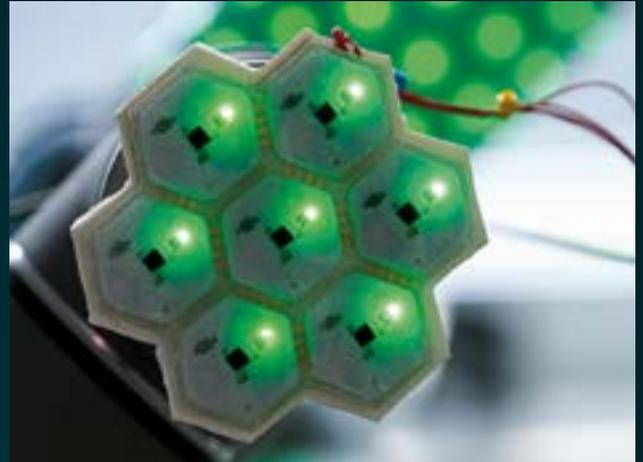
Each hexagonal cell of the artificial skin comprises four sensors that measure pressure, proximity, temperature and vibration as indications for touch. The interconnected cells pass electrical signals via varied pathways through the entire skin to and from the central computer.
