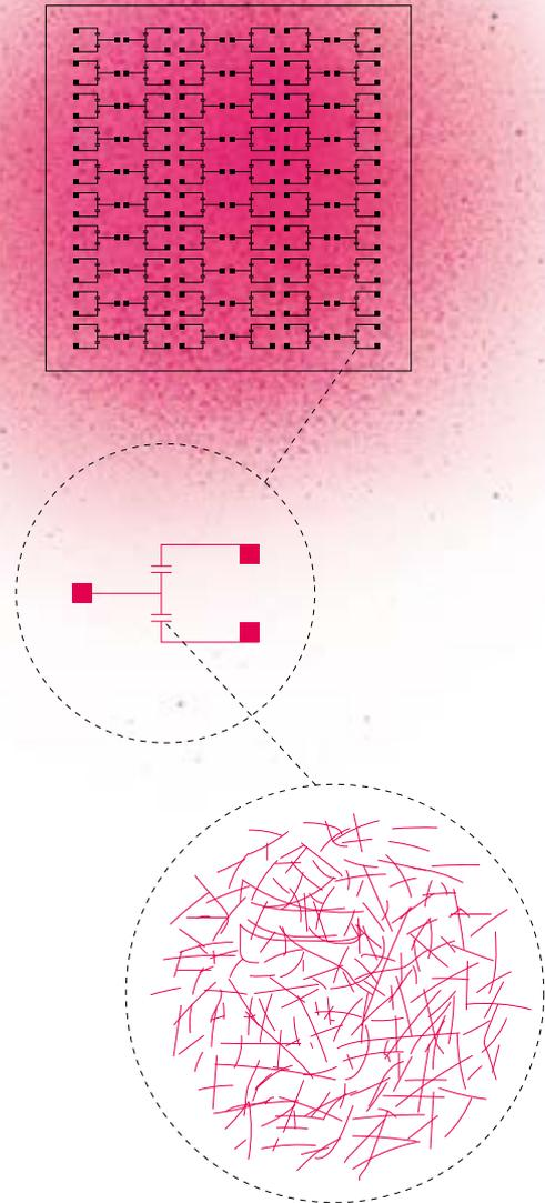
**When viewed under the microscope** we can see that the structures of the sensors (center) are composed of extremely fine carbon nanotubes (bottom) that form a dense mesh when deposited onto a surface. With their spray method, the TUM researchers can layer them onto films in large quantities (top).
