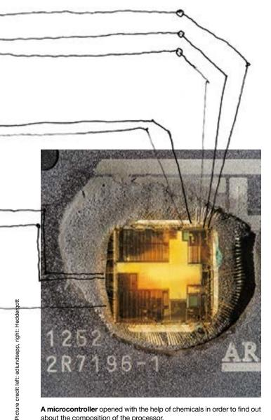
A microcontroller opened with the help of chemicals in order to find out about the composition of the processor.
