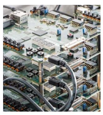
**Connected evaluation boards** with field programmable gate arrays are used to test out ideas for new PUFs.
