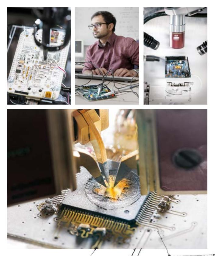
Chips under attack in Georg Sigl's laboratory: Measuring electromagnetic radiation to prepare for side channel attacks (top left); fault injection with power glitches in order to perform fault attacks (top center); firing laser beams at an open processor chip while it carries out calculations. The laser causes calculation failures, which can be used to extract secret information (top right). Side channel attack by means of three highly sensitive measuring probes (bottom).
