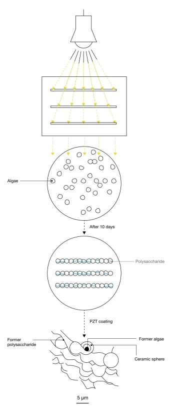
**Finest structures created by algae:** Light guides the growth of red microalgae, which secrete polysaccharides during the process. The researchers have managed to coat these structures with lead zirconium titanate (PZT), a piezoelectric ceramic. The formations are then heated to 500-600°C to eliminate all organic matter. The result is a structure made of hollow ceramic spheres
